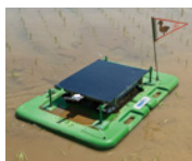
“Aigamorobo” automatic weed inhibitor robot Inhibits weed germination in rice paddies
